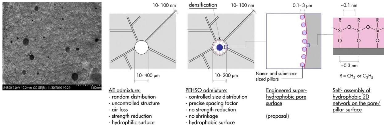
**Fig. 4: How the Superhydrophobic Hybridization of Concrete Works**
