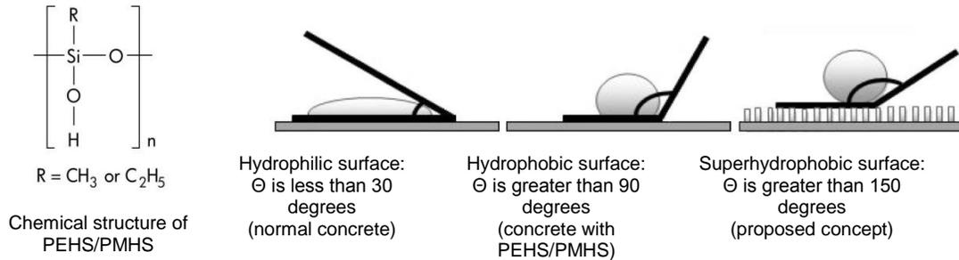
**Figure 3: The Concept of Superhydrophobic Hybridization of Concrete Pore Surface**
