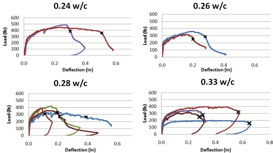
**Figure 2: Load vs. deflection of flexural tests for PVA fibers in ECC.**
