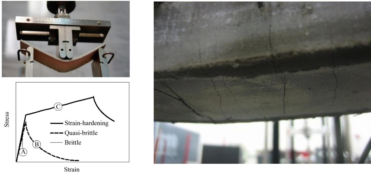
**Figure 1: The Strain-Hardening Performance of ECC**
